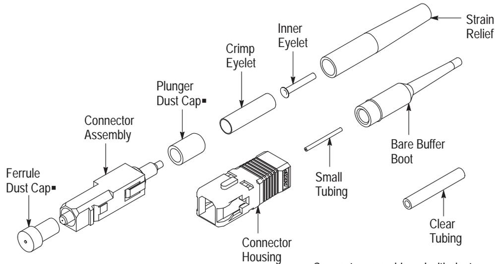
▪ Connectors are shipped with dust caps installed onto connector. Keep dust caps in place until ready for assembly.
